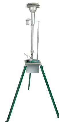
PQ100 Ambient PM<sub>10</sub> Sampler
